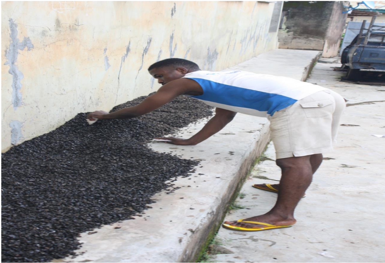
Plate 2.2: Spreading and sun-drying of PKS
