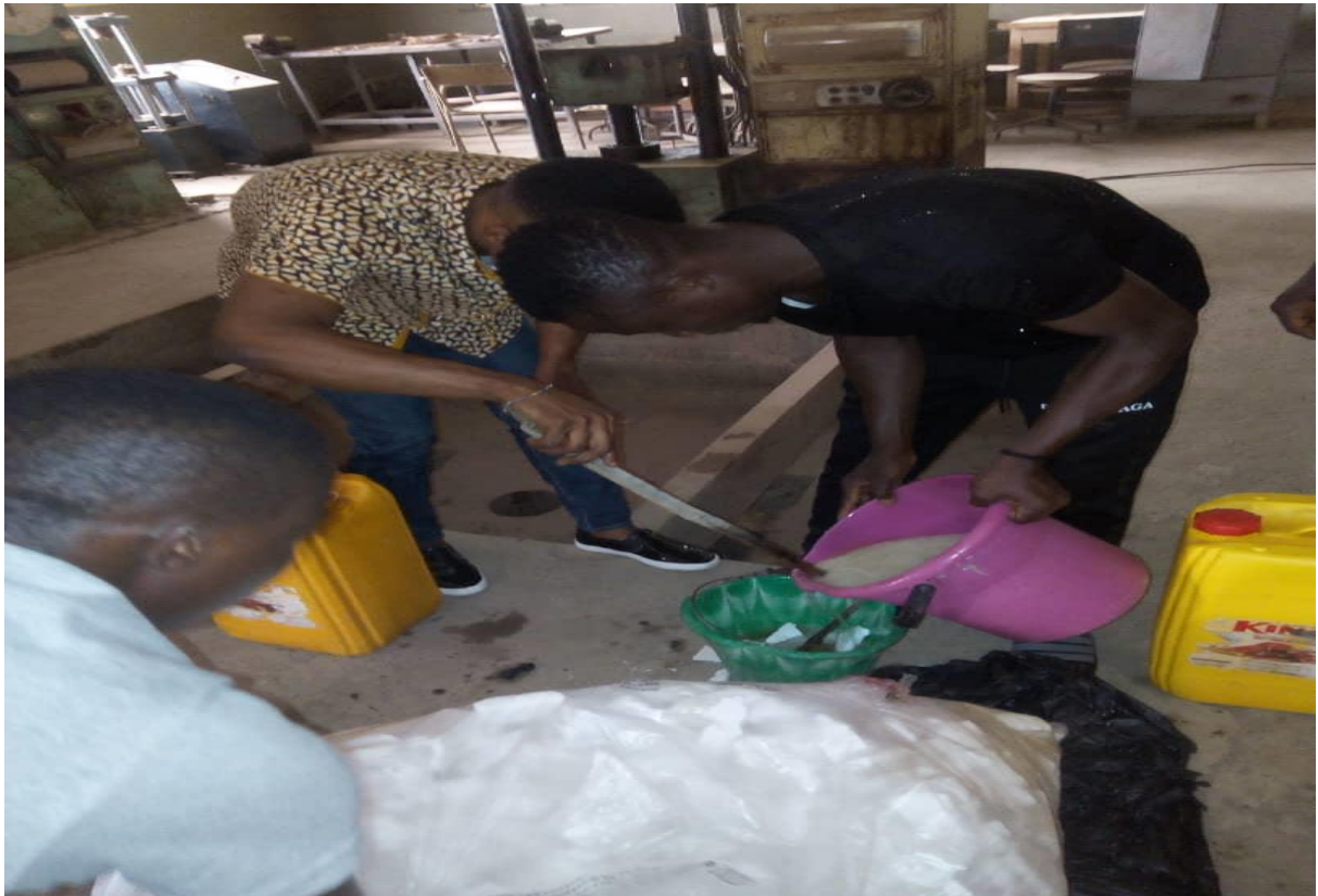
Plate 2.6: Production of polystyrene paste (polystyrene plus petrol)
