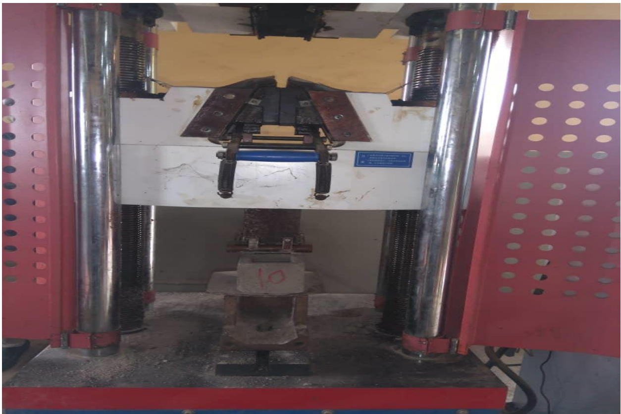
Plate 3.10: Block sample under flexural load
